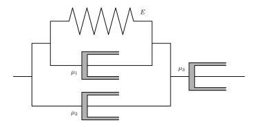
Derive the stress-strain relation for this element.
