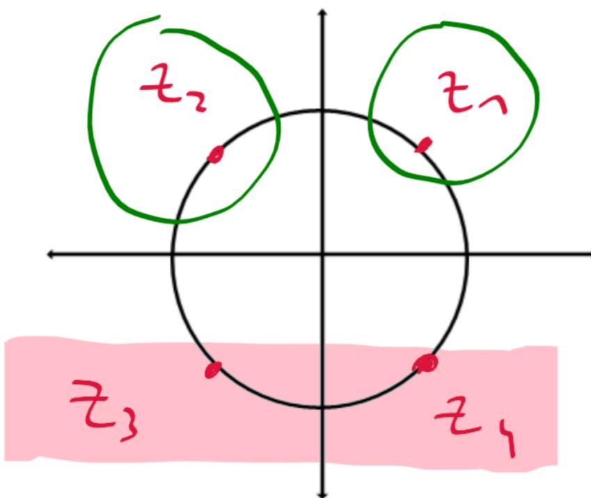
$$\begin{aligned} z^4 + 1 &= 0 \\ z^4 &= -1 \\ z &= \sqrt[4]{-1} \end{aligned}$$
