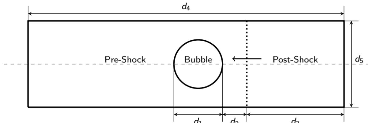
Figure: A schematic of the computational domain for shock-bubble interaction problem.
