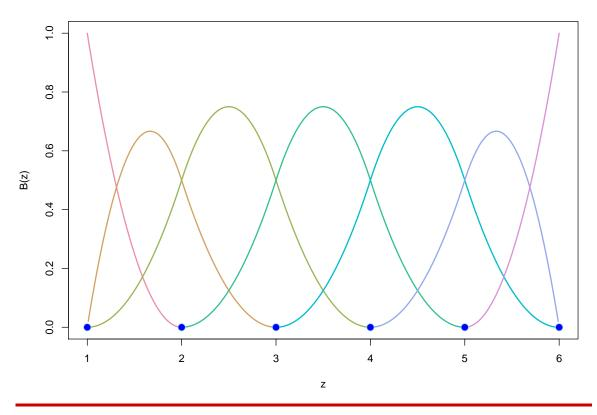
Cubic B-spline basis (of degree d = 3)
