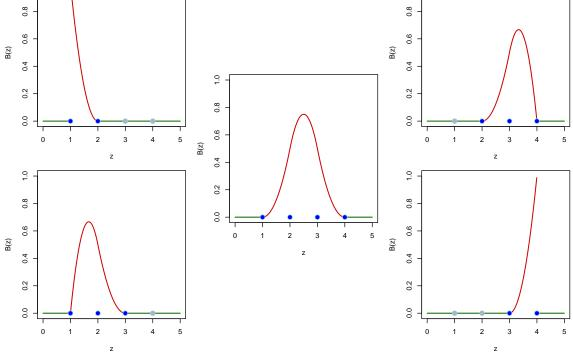
Some basis splines of degree d = 3 with possibly coincident boundary knots
