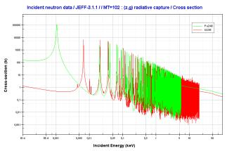
Radiative capture cross sections of <sup>238</sup>U and <sup>240</sup>Pu
