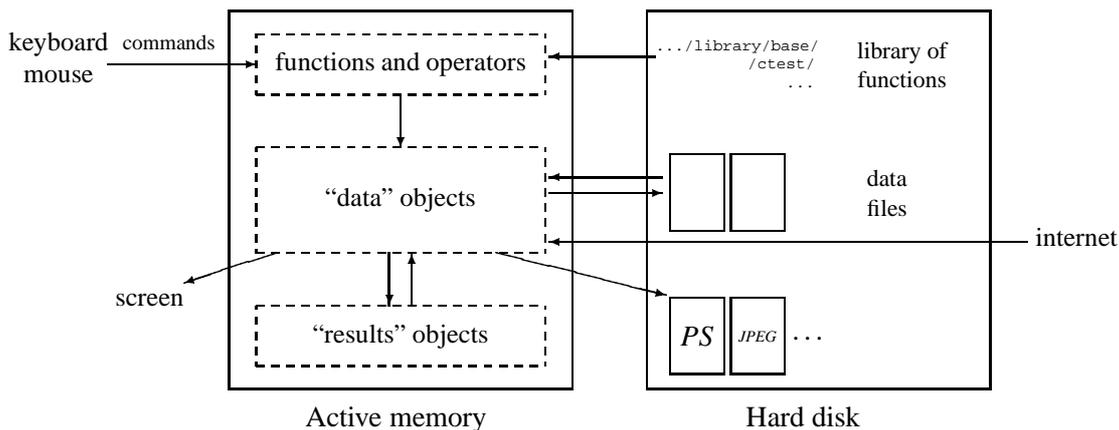
Figure 1: A schematic view of how R works.
