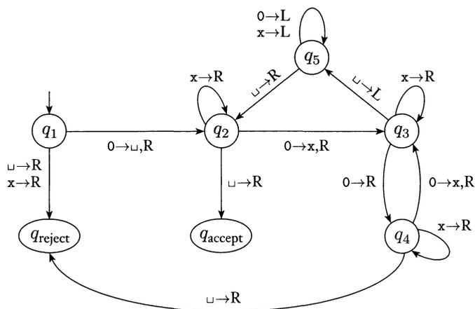
FIGURE 3.8 State diagram for Turing machine  $M_2$
