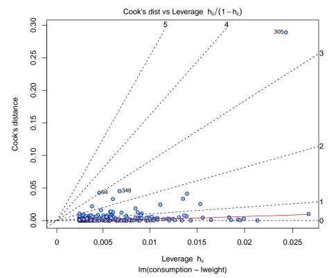
The x-axis shows values of  $h_{i,i}/(1-h_{i,i})$  and not  $h_{i,i}$ . Contours are related to the values of  $U_t^{std}/\sqrt{k}$ .
