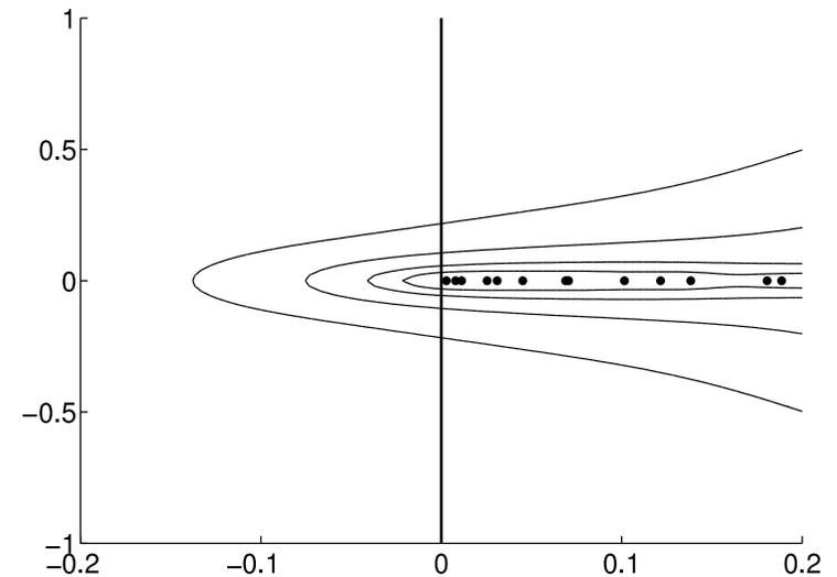
Development of the “test quantity”  $|(v_h, v_h^*)|$  under mesh refinement for the critical eigenvalues of the linearized (about Couette flow) Navier-Stokes operator with Neumann inflow conditions for different Reynolds numbers  $Re = 100, 350, 500, 1000, 3500, 5000, 10000$ .
