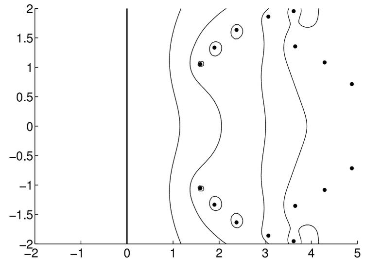
Pseudospectra of the linearized (about Couette flow) **Burgers (left)** and **Navier-Stokes operator (right)** with Neumann inflow conditions for  $\nu = 0.01$ : The dots represent eigenvalues and the lines the boundaries of the  $\epsilon$ -pseudospectra for  $\epsilon = 10^{-1}, \dots, 10^{-4}$ .
