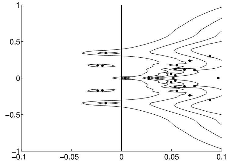
Development of the “test quantity”  $|(v_h, v_h^*)|$  under mesh refinement for the critical eigenvalues of the linearized (about the channel flow) Navier-Stokes operator with Neumann inflow conditions for different Reynolds numbers  $\text{Re} = 20, 40, 45, 50, 60$  and increasing level of refinement.
