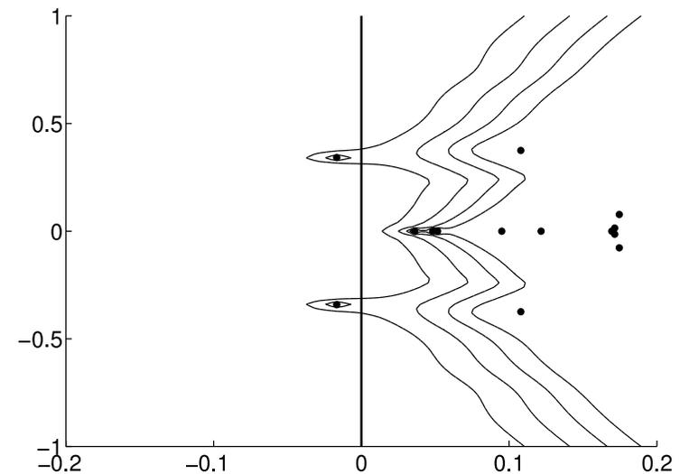
Development of the “test quantity”  $|(v_h, v_h^*)|$  under mesh refinement for the critical eigenvalues of the linearized (about the channel flow) Navier-Stokes operator with Dirichlet inflow conditions for different Reynolds numbers  $\text{Re} = 20, 40, 45, 50, 60$  and increasing level of refinement.
