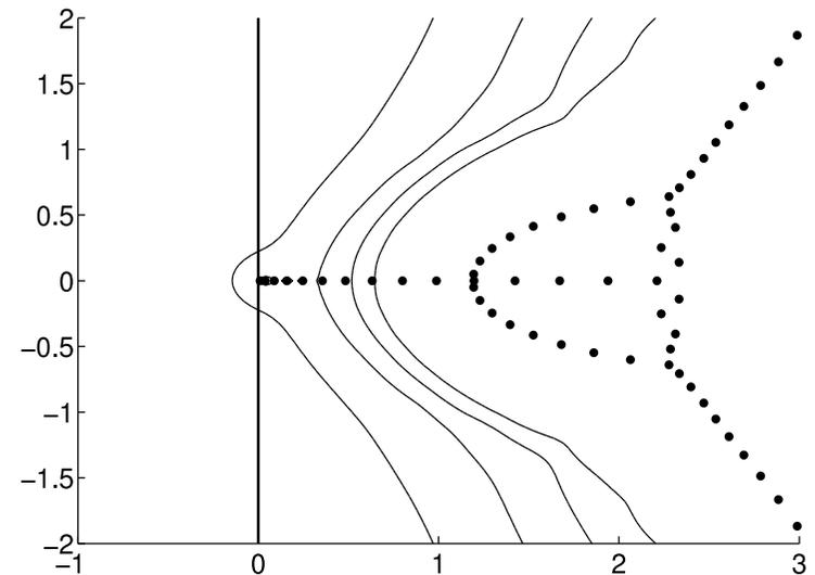
Pseudospectra of the linearized (about Couette flow) **Burgers (left)** and **Navier-Stokes operator (right)** for  $\nu = 0.01$  and Dirichlet inflow condition: The dots represent eigenvalues and the lines the boundaries of the  $\epsilon$ -pseudospectra for  $\epsilon = 10^{-1}, \dots, 10^{-4}$ .
