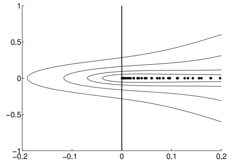
Development of the “test quantity”  $|(v_h, v_h^*)|$  under mesh refinement for the critical eigenvalues of the linearized (about Poiseuille flow) Navier-Stokes operator with Neumann inflow conditions for different Reynolds numbers  $\text{Re} = 100, 350, 500, 1000, 3500, 5000, 10000$ .
