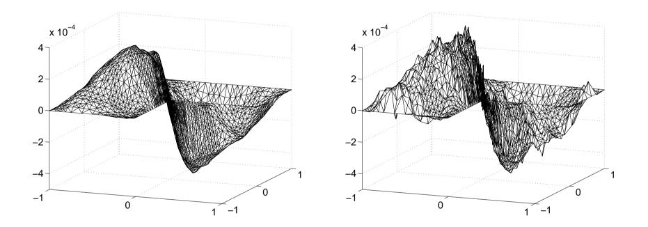
Algebraic error  $x_h - x_h^{(n)}$  (left) and the total error  $x - x_h^{(n)}$  (right) after the number of CG iterations guaranteeing
