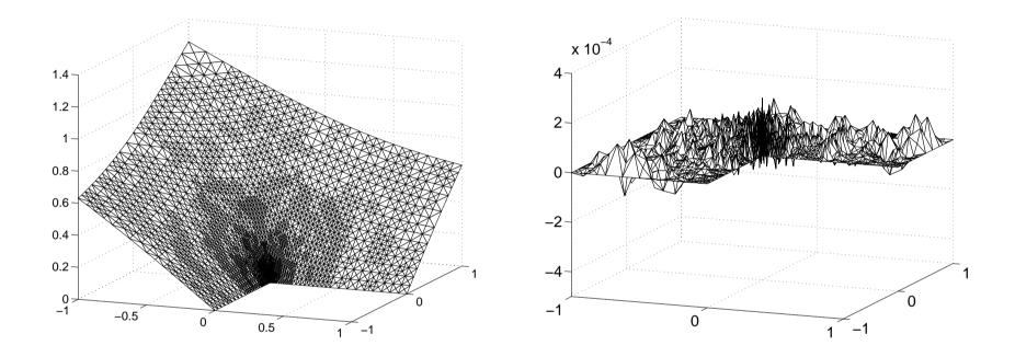
Exact solution x (left) and the discretisation error  $x - x_h$  (right) in the Poisson model problem, linear FEM.
