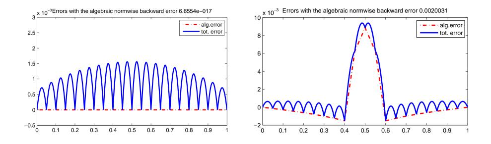
The discretisation error (left), the algebraic and the total error (right),
