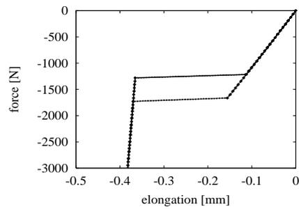
Fig. 1b Loading/compression curve of a  $Ni_2MnGa$  single crystal at  $\theta = 50^\circ C$ .
