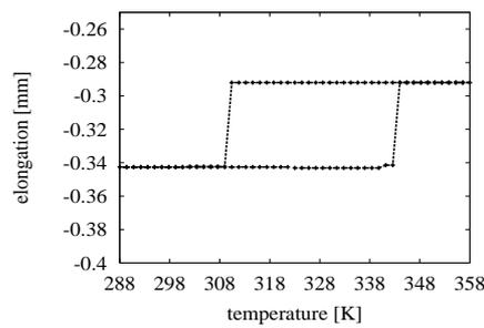
Fig. 2 The specimen under the load of  $-200 MPa$  is heated up and then cooled down. A hysteretic response of the temperature vs. elongation.
