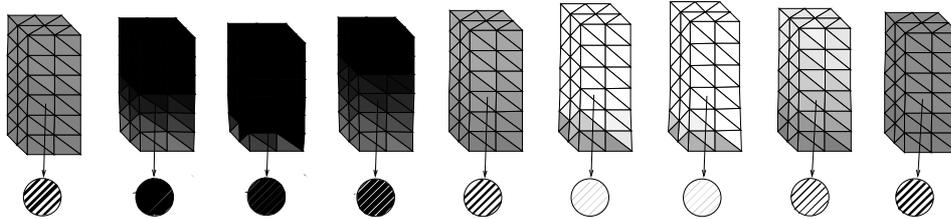
Fig. 5 Evolution of a martensitic reorientation during quasi-plastic cycling at  $\theta = 20^\circ\text{C}$  showing martensitic variants  $U_2$  (black) and  $U_3$  (white) in the specimen during the loading cycle. Evolving microstructure with the normal of laminates  $(1, 1, 0)$  is depicted on one element. The displacement is displayed as magnified by the factor 2. The specimen is here discretized into 120 elements.
