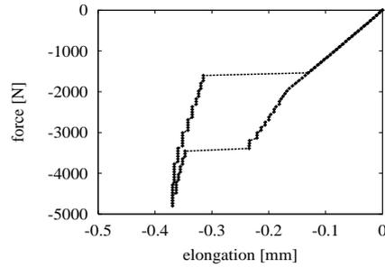
Fig. 4 Pseudo-elastic stress-strain response under the compression test during the loading cycle from Fig. 3.
