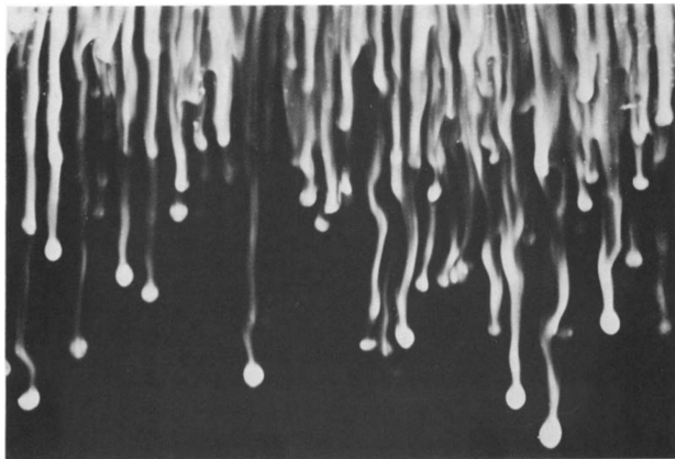
FIGURE 1. A field of salt fingers formed by setting up a stable temperature gradient and pouring a little salt solution on top. The downward-moving fingers were made visible by adding fluorescein to the salt and lighting through a slit from below.
