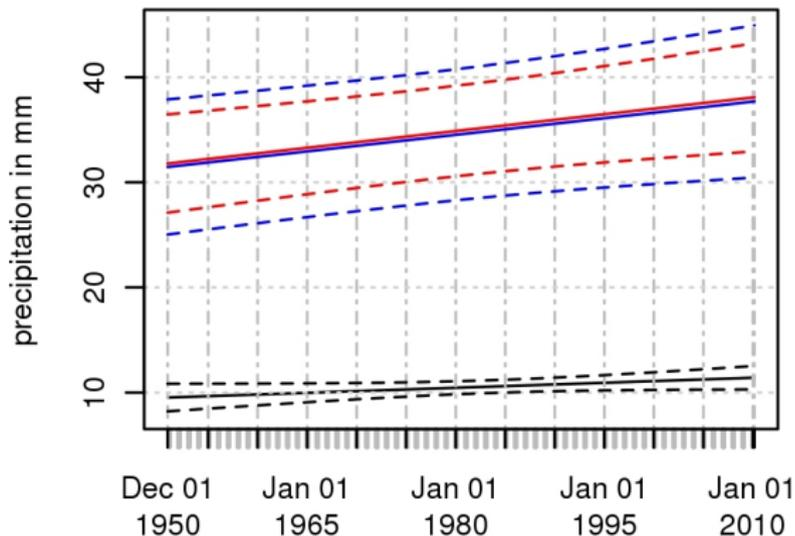
Estimated threshold with 95% pointwise confidence band (black) and 25-year return level based on the at-site estimation (blue) and the IF approach (red), together with pointwise confidence bands, for the grid box around De Bilt.
