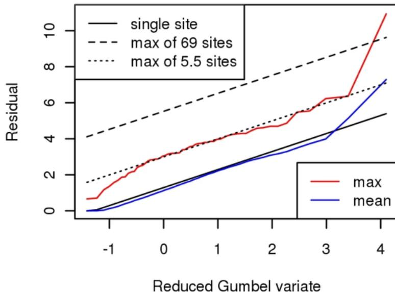
Spatial mean Gumbel plot (blue), Gumbel plot of the maxima over the grid (red) and theoretical distributions for the maximum of a different number of Gumbel variables (black)
