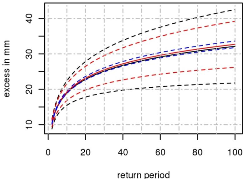
Estimated return levels of the excesses (solid lines) with 95% pointwise confidence bands (dashed lines) for the year 1980 at the grid box around De Bilt (black – site-specific, red – IF, blue – no correction of the standard error for spatial dependence)
